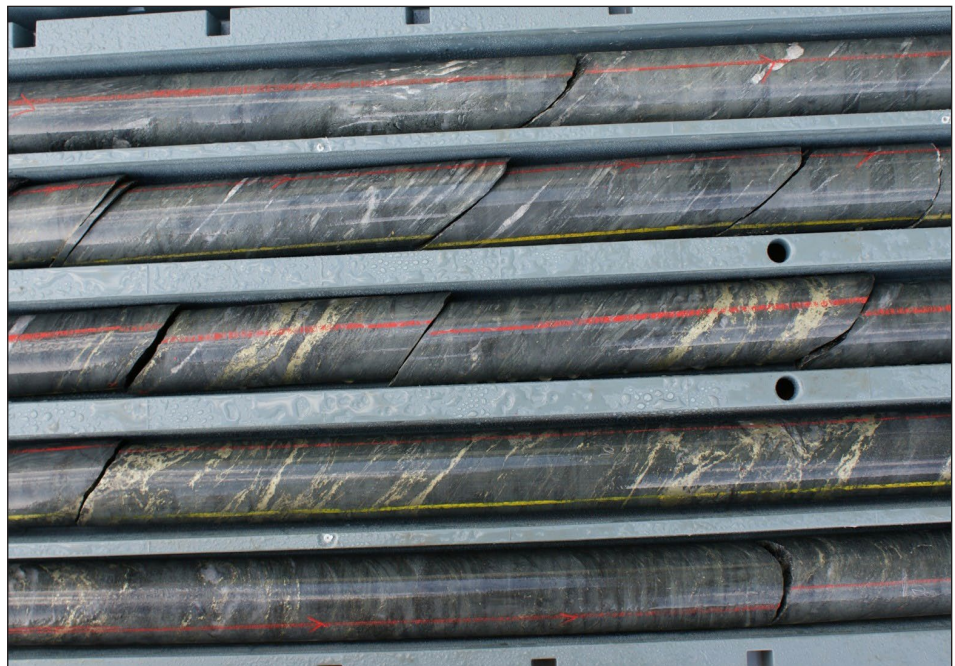
Figure 12: Disseminated and vein-fill chalcopyrite, ~275 m downhole, CAND001 - core diameter is ~45 mm
