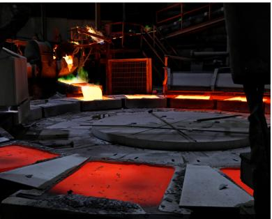
View of the anode copper casting and molds in the smelting plant
